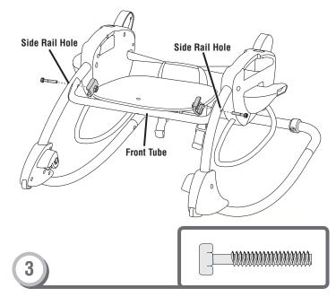
Insert a M5 x 2,9 cm screw through the outside of each side rail and into the ends of the front tube.
